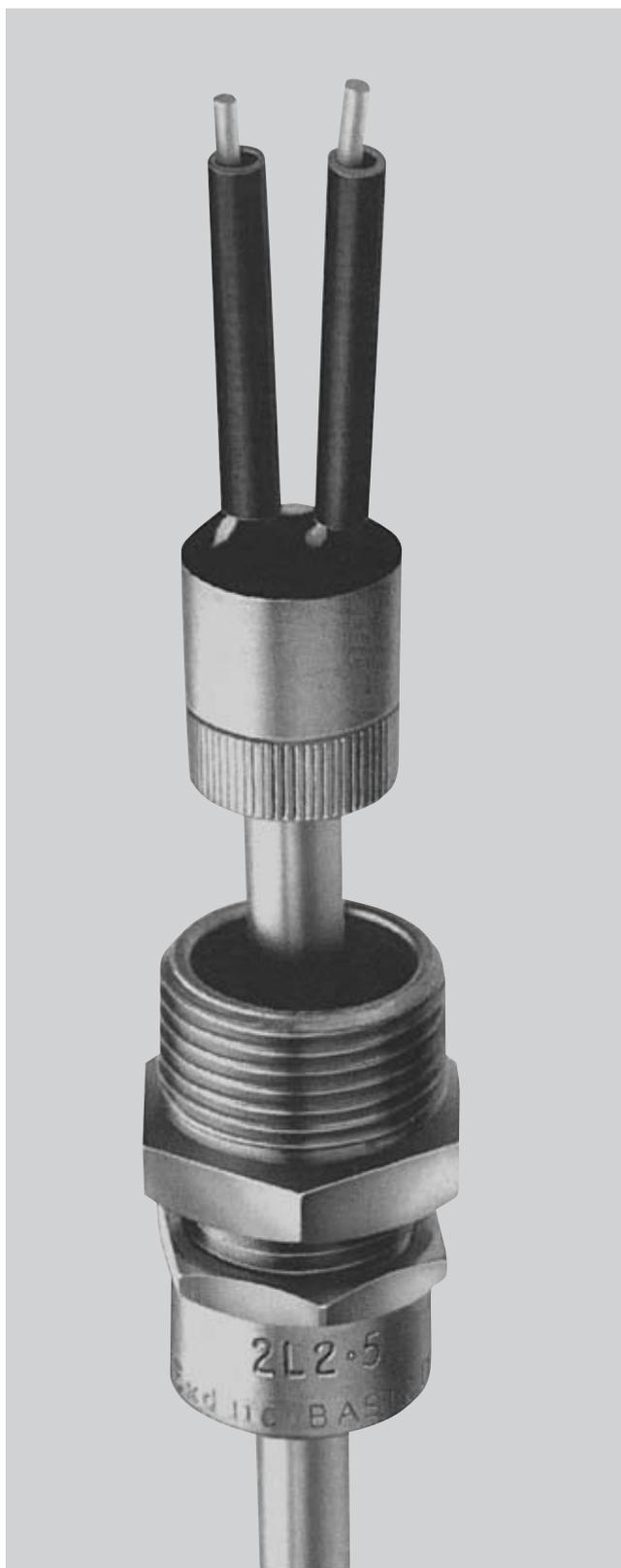
The insulator consists basically of a brass screw-on pot with a glass filling medium and is suitable for use at temperatures between 150°C and 250°C.
